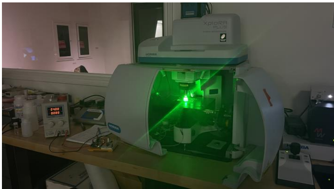
Raman Spectroscopy to determine Pb uptake properties in crystal
