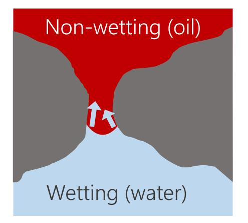
Wetting fluid enters the narrowest pores first
