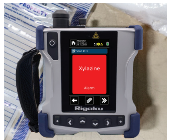
The Rigaku CQL Narc-ID™ 1064 nm Raman analyzer displaying a result for xylazine.
