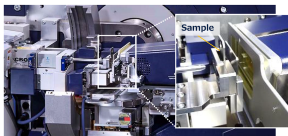
Fig. 4. Transmission 2D-WAXS optical system (camera length 27 mm).
