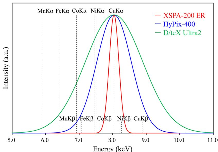
Fig. 1. The energy distribution of three detectors calculated using the energy resolution for the  $\text{CuK}\alpha$  line, and the fluorescent X-rays energy of each element.
