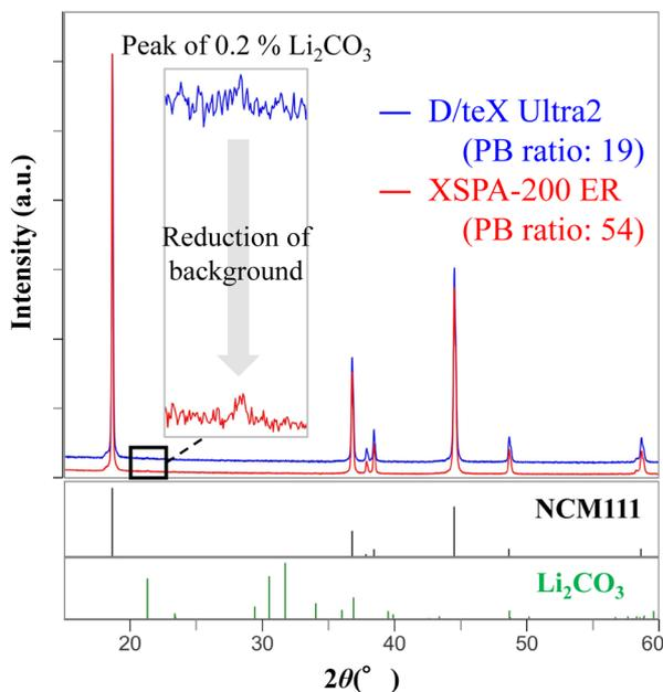
Fig. 2. Comparison of XRD patterns of NCM111 measured by two different detectors.
