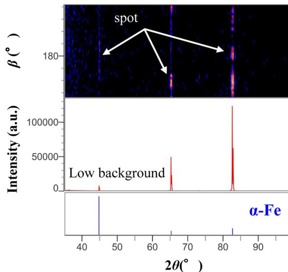
Fig. 3. 2D measurement data of steel material.
