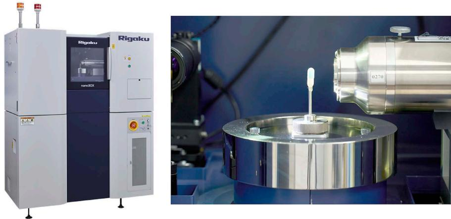
Fig. 1. Laboratory-based X-ray microscope, nano3DX. External appearance (left) and region around sample stage (right).
