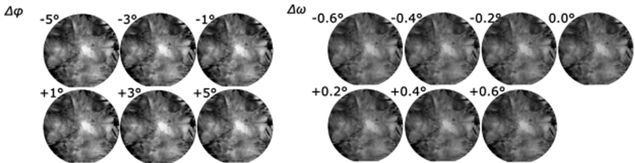
Fig. 2. XRT images of the 1120 reflection of a 150-mm 4H-SiC wafer taken at various  $\phi$  (azimuthal angles) and  $\omega$  (incident angles).
