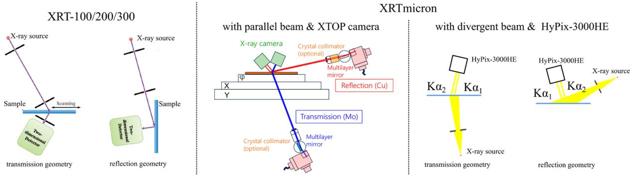
Fig. 1. Schematic images of XRT systems launched by Rigaku.<sup>(1)</sup>
