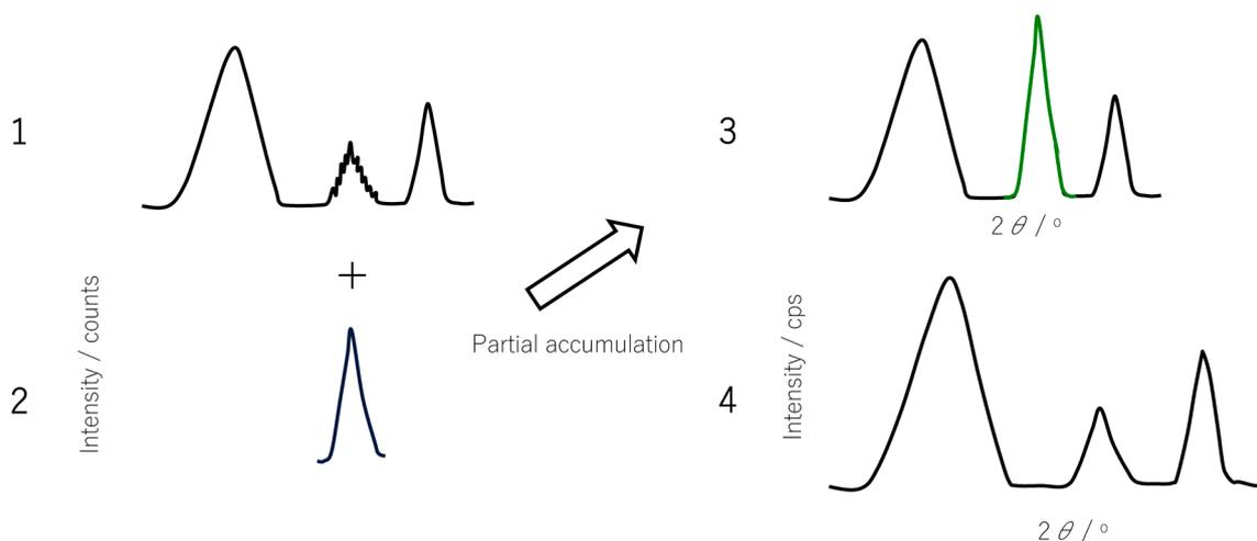
Fig. 1. The schematic diagram of partial accumulation measurement.
