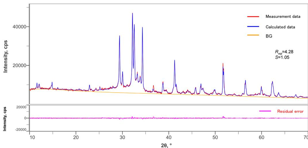
Fig. 4. Rietveld refinement result of the blast furnace slag cement.
