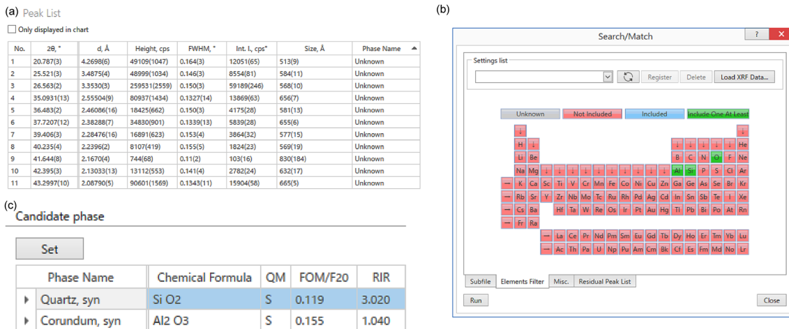
Fig. 4. Procedure of phase identification by SLSII. (a) Peak list, (b) Conditions example for search/match, (c) candidate phase list.
