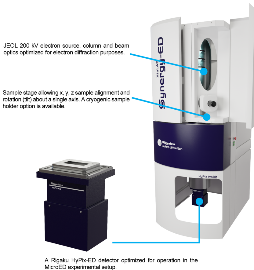
Fig. 3. Hardware components of the Synergy-ED.
