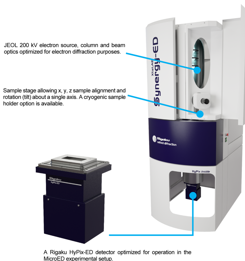
Fig. 3. Hardware components of the Synergy-ED.
