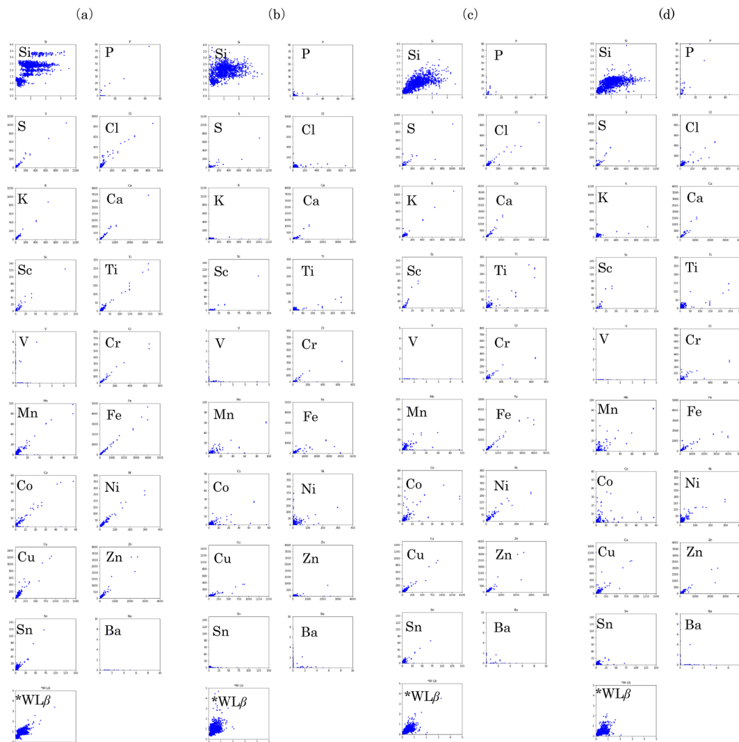
Fig. 5. Correlation plots of analyzed results measured by TXRF-V310. X-axes: 60-second measurement results, Y-axes: 5-second measurement results by (a) Conventional method, (b) ML1, (c) ML2 and (d) ML3. ML1, ML2 and ML3 are mentioned in detail in Subject. 3.1.
