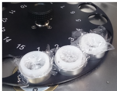
Fig. 6. Organic solvents measured by NEX CG.
