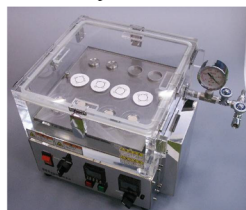
Fig. 4. (a) UltraCarry, for hazardous heavy elements and some light elements. Sample should be pipetted on the special paper in the center. (b) UltraCarry Light, for a wide range of elements. (c) UltraDry, the dedicated vacuum dryer. It can be used for vacuum drying and low-temperature heating. Drying time is about 30 minutes (depends on the number of samples).
