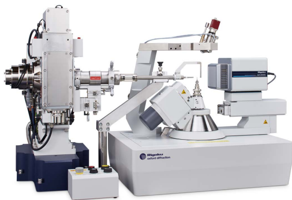
Fig. 8. XtaLAB SynergyCustom with FR-X high flux X-ray source and HyPix-6000HE detector.
