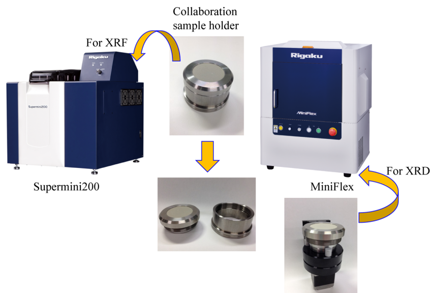
Fig. 11. Configuration of the collaboration sample holder for benchtop XRD and XRF instruments.
