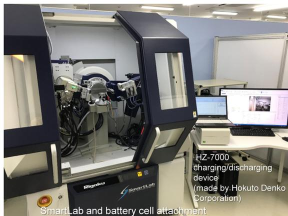
**Fig. 7.** Battery evaluation system consisting of SmartLab X-ray diffractometer and HZ-7000 charging/discharging system.
