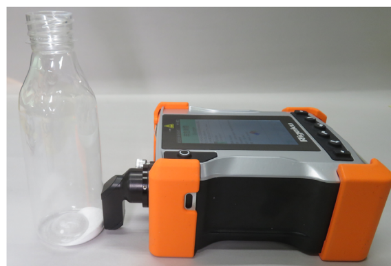
Fig. 14. Periscope adaptor for small amount at the bottom.
