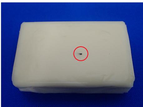
Fig. 12. A piece of metal in a block of cheese.
