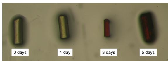
**Fig. 5.** Changes in crystalline sponge color with soaking time when trapping cypress essential oil.
