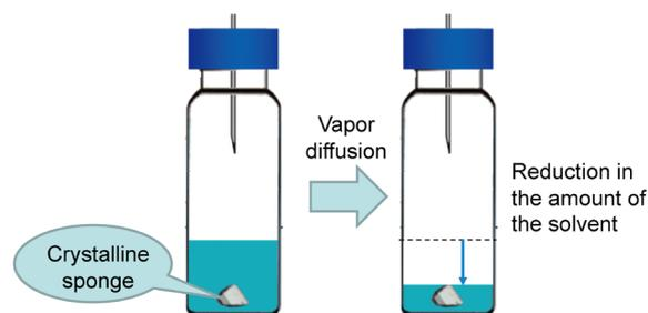
Fig. 3. Previous soaking procedure: The solvent gradually evaporates through the injection needle mounted on the cap of the vial.
