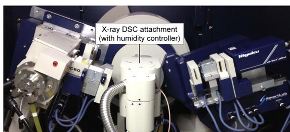
Fig. 2. X-ray diffractometer equipped with an X-ray DSC attachment.
