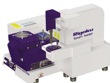
Fig. 1. TG 8121 with sample observation attachment and an auto sample changer.
