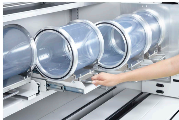
Fig. 3. Vacuum path changing system.
