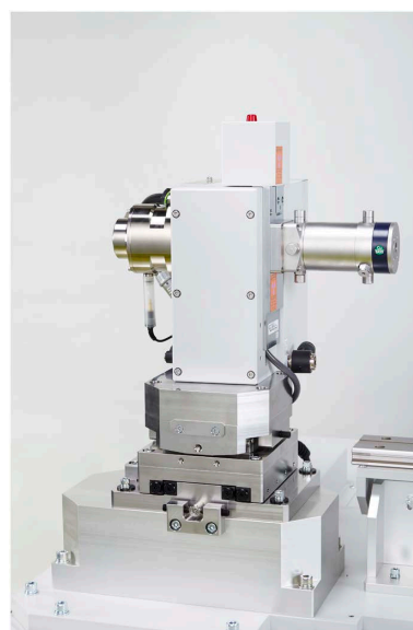
Fig. 1. Appearance of beam module (MicroMax007HFMR and OptiSAXS confocal multilayer mirror).
