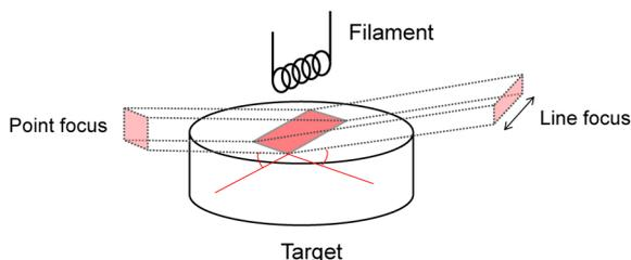
Fig. 2. Geometrical configuration of take-off directions for point focus and line focus.
