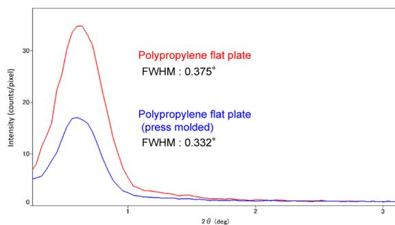
**Fig. 19.**  $2\theta$ - $I$  profile of polypropylene flat plates.
