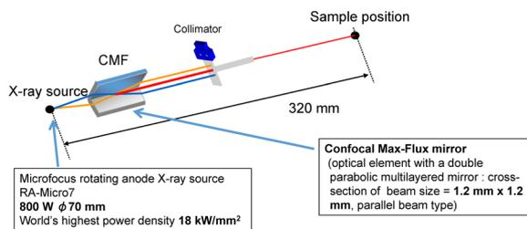
Fig. 3. Example of incident optical system configuration of SmartLab  $\mu$ HR.
