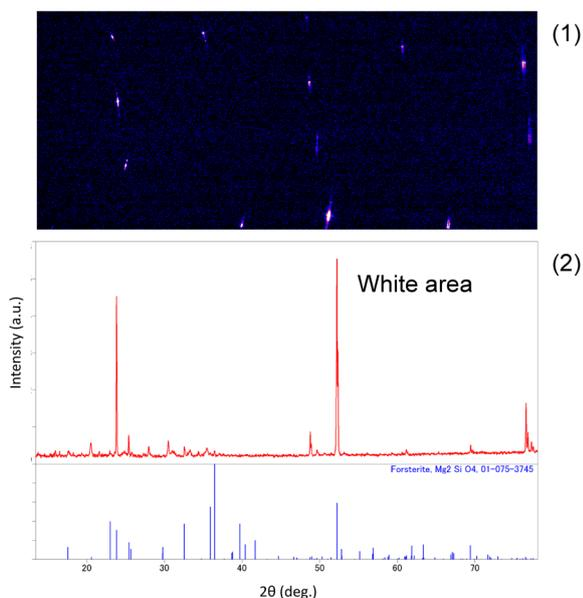
Fig. 12. (1) Two-dimensional diffraction image of white area by measurement with oscillation.
