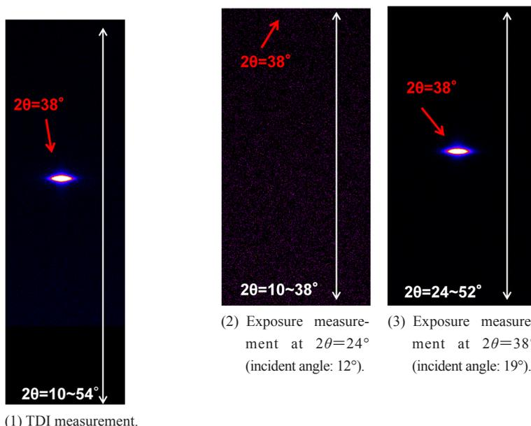
Fig. 7. TDI ( $2\theta/\theta$ ) measurement and exposure ( $2\theta$ ) measurement of Au thin film on Si substrate.
