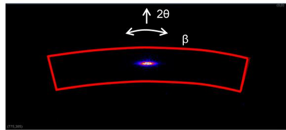
Fig. 8. Two-dimensional diffraction image of 111 reflection of Au thin film on Si substrate.
