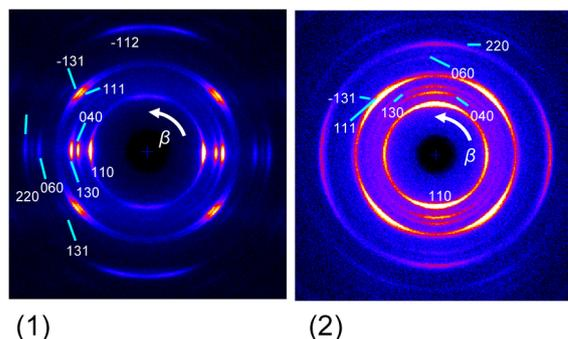
Fig. 14. Result of 2D-WAXS measurement of uniaxially and biaxially stretched polypropylene film.
