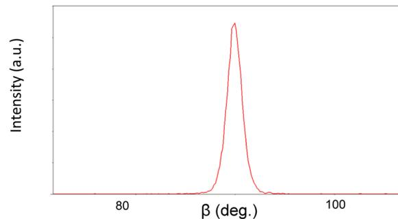
Fig. 9.  $\beta$ - $I$  profile of 111 reflection of Au thin film on Si substrate.
