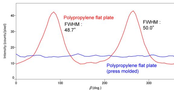
**Fig. 18.**  $\beta$ - $I$  profile of polypropylene flat plates for long-range order peak.
