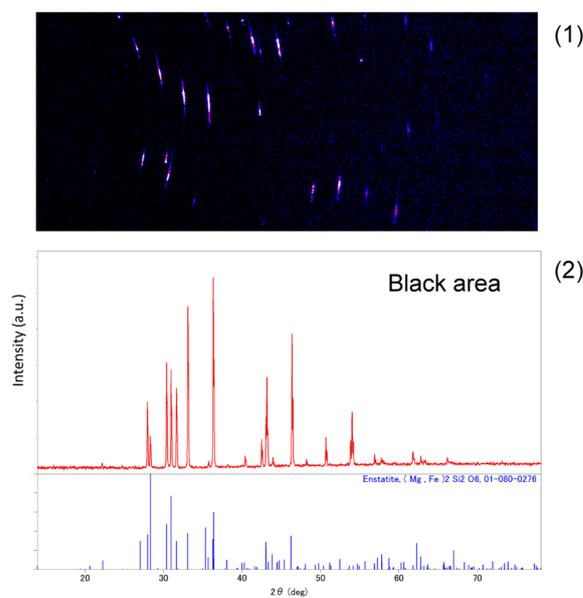
Fig. 13. (1) Two-dimensional diffraction image of black area by measurement with oscillation.
