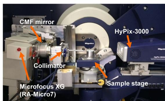
Fig. 1. SmartLab  $\mu$ HR.
