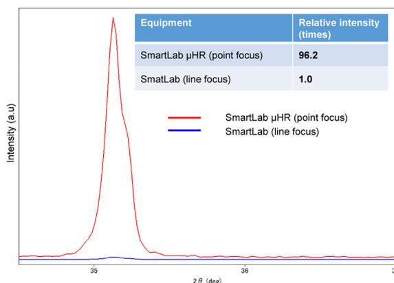
Fig. 4. Comparison of intensity between SmartLab and SmartLab  $\mu$ HR.
