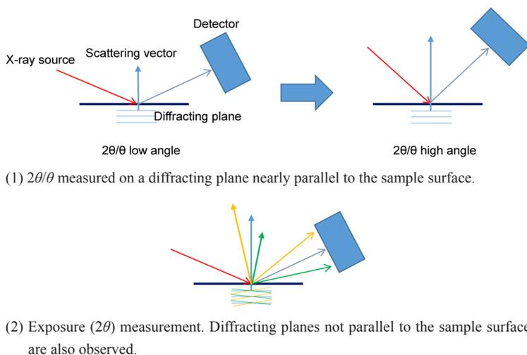
Fig. 6. Schematic drawing of  $2\theta/\theta$  and  $2\theta$  (exposure) measurement using 2D detector.
