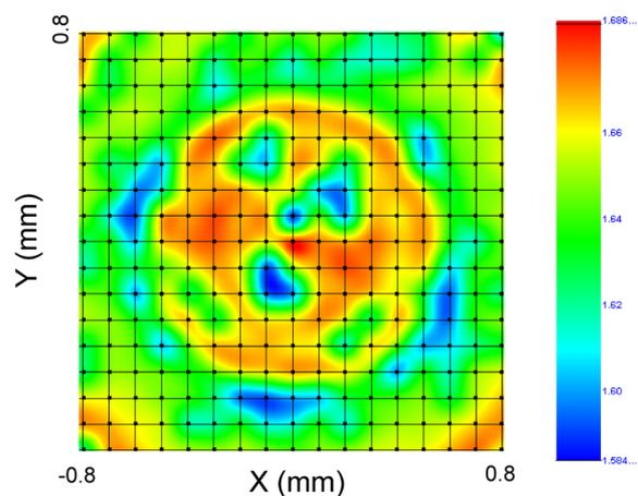
Fig. 10. Result of peak width distribution analysis for mapping data of 111 reflection of Au thin film on Si substrate.
