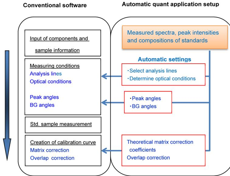
Fig. 1. Setting parameters in the new “ZSX Guidance” for quant application setup.
