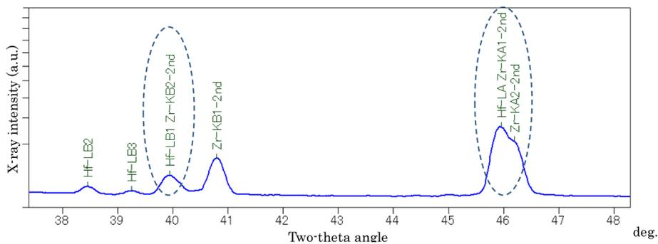
Fig. 4. Qualitative chart of Hf-L $\alpha$  and Hf-L $\beta_1$ . Analyzing crystal: LiF (200), Detector: SC
