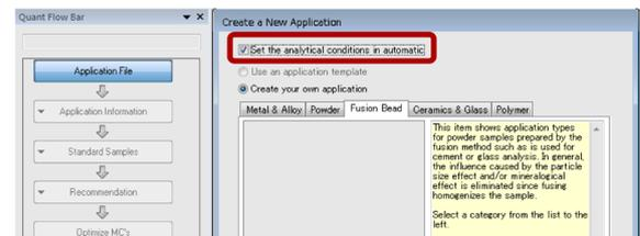
Fig. 2. Initiate “Automatic quant setting”.
