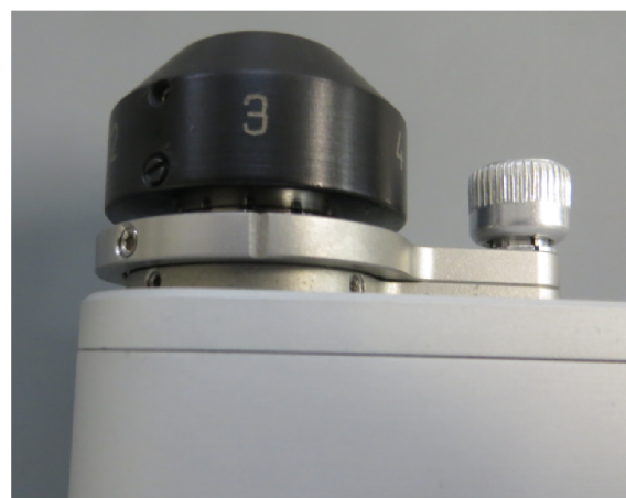
Fig. 2. Adjustable focal point nose cone.
