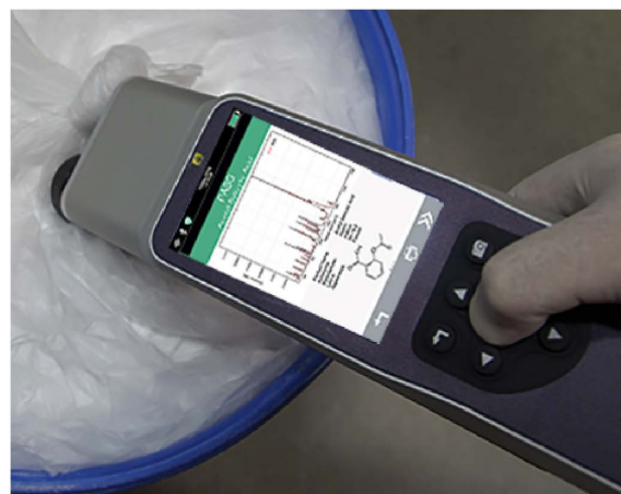
Fig. 1. Handheld Raman spectrometer Progeny.
