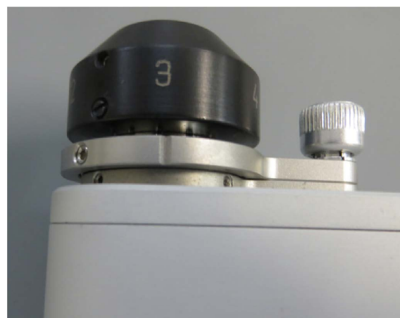
Fig. 2. Adjustable focal point nose cone.
