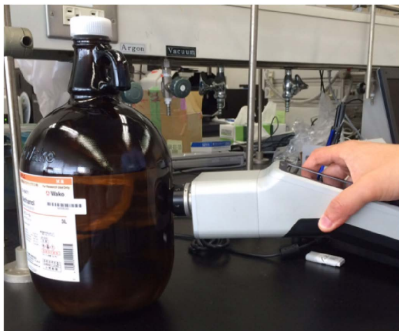
Fig. 3. Analysis of liquid contained in a glass bottle.
