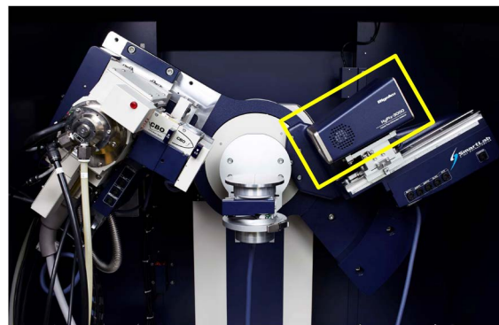
Fig. 1. SmartLab intelligent X-ray diffraction system equipped with HyPix-3000 hybrid multi-dimensional pixel detector.
