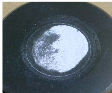
Fig. 11. Titanium oxide powder stuck to die after pelletization
