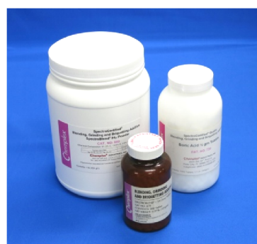
Fig. 7. Binder for pelletization (Spectro Blend ® ).
