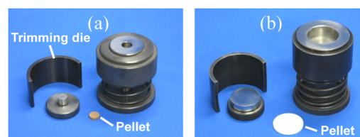
Fig. 5. Sample preparation with cylinder type dies.
