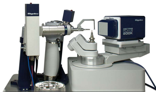
Fig. 3. The standard configuration of the XtaLAB PRO series includes a PILATUS 200K detector, a kappa goniometer, a Cu microfocus sealed tube source (MicroMax-003) and a 3 kW Mo sealed tube source.
