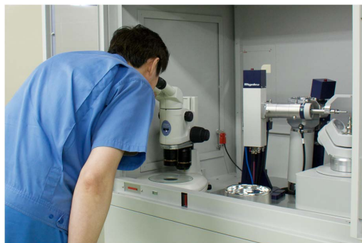
Fig. 10. There is enough room inside the XtaLAB PRO enclosure to place items that can be useful in mounting sensitive crystals quickly.
