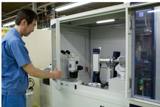
Fig. 9. The XtaLAB PRO enclosure was designed to allow maximum access to the instrument.
