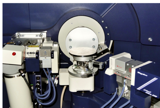
Fig. 4. Unique in-plane axis drives detector in a plane parallel to sample surface, which enables to see in-plane lattice parameters, crystal structure as a function of depth from the sample surface.
