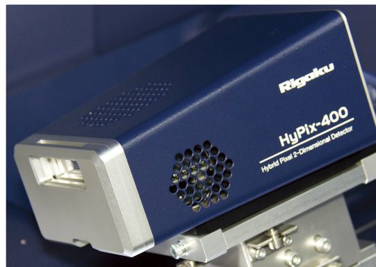
Fig. 3. HyPix-400, a 2-dimensional detector based on semiconductor hybrid pixel array detector (HPAD) technology.
