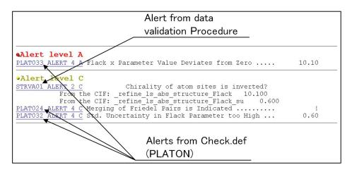
Fig. 6. Output when the value of \_refine\_ls\_abs\_structure\_Flack was set to 10.1 and reliability was set to 0.6.
