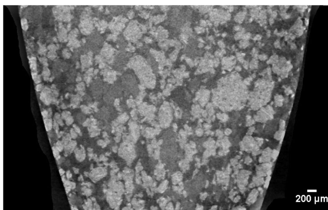
Fig. 11. Reconstructed CT image of a dietary supplement tablet (includes Mg, Ca and Zn).
