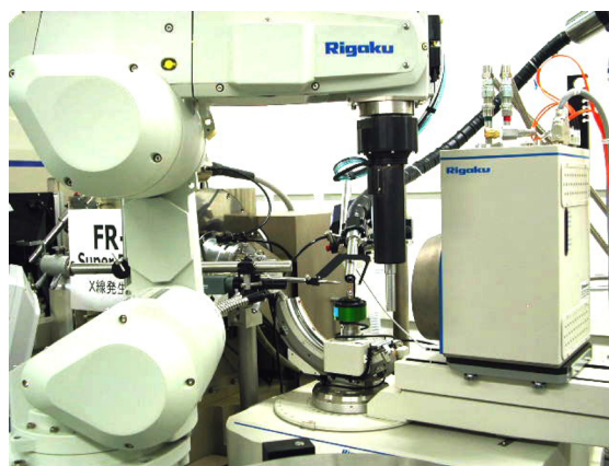
Fig. 6. A high-throughput single crystal X-ray structure analysis system. A sample changer, automated crystal centering and evaluation are integrated. This system gives us options such as data collection in the descending order of the score and elimination of crystals below a threshold.
