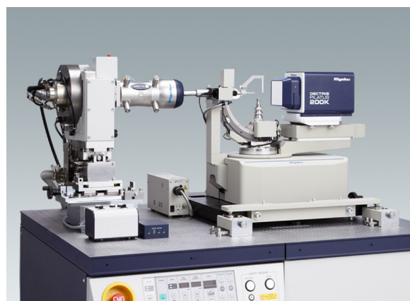
Fig. 4. An XtaLAB P200 system consists of a hybrid pixel array detector (PILATUS 200K), a dual wavelength microfocus X-ray generator (MicroMax007HF-DW) and a multilayer optics (VariMax DW).
