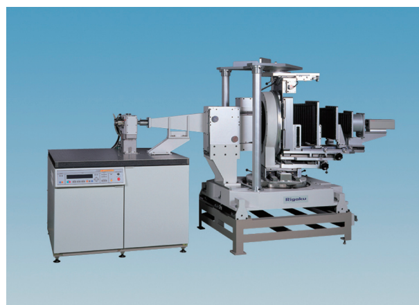
Fig. 9. Conventional topography system for 300-mm wafers.
