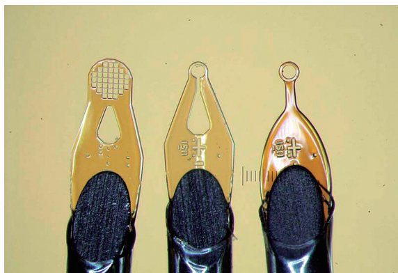
Fig. 1. MiTeGen pins. MicroMesh (left) is used for micro or thin crystals. The one in the center is the original MicroMount. MicroMount LD (right) was developed for small molecule crystals.
