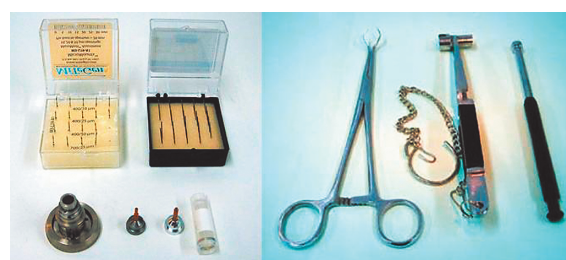
Fig. 7. Typical tools for low temperature measurement. From front left to right in the left picture: a goniometer head with a magnetic base, goniometer bases (MiTeGen and Hampton Research), cap for the bases. Upper left to right, MicroMount (MiTeGen) and CryoLoops (Hampton Research). The right picture includes tools used for freezing by liquid nitrogen and storing crystals at liquid nitrogen temperature. From left to right, Vial Clamp, CryoTong and CrystalWand (Hampton Research).
