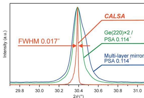
Fig. 1. Comparison of profiles for LaB<sub>6</sub> 110 diffractions. The profiles are normalized with each peak height.
