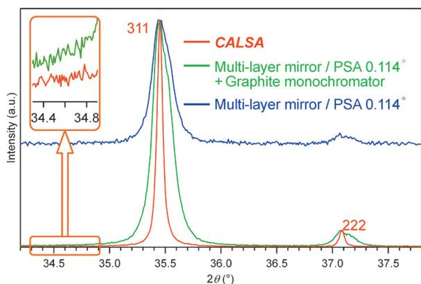
**Fig. 2.**  $\text{Fe}_3\text{O}_4$  (magnetite) diffraction patterns of 311 and 222 diffraction peaks. The intensities are normalized by 311 diffraction peak heights.
