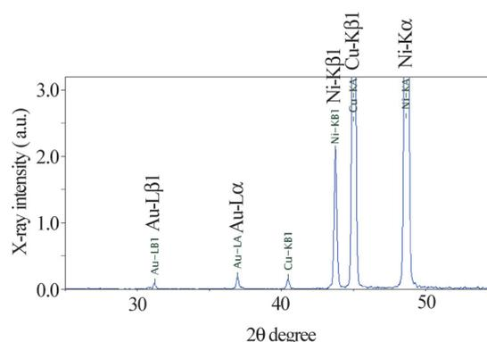
Fig. 6. XRF spectrum for the gold-coated terminal.
