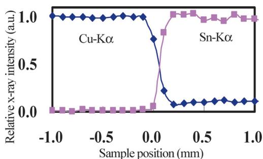
Fig. 4. Spatial-resolution test results (knife-edge scan).
