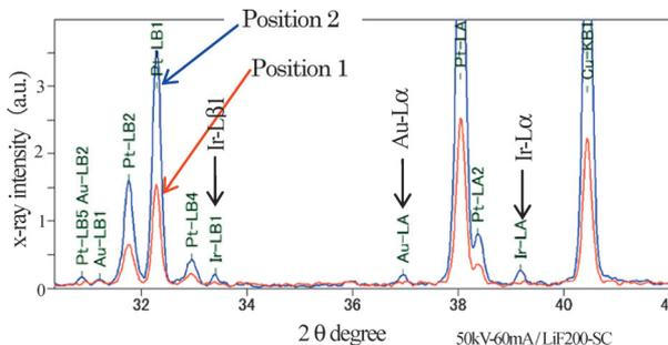
Fig. 11. XRF spectra obtained from positions 1 and 2.
