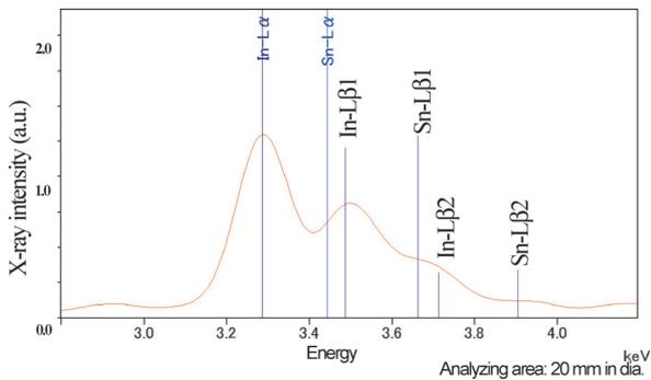
Fig. 9. EDXRF spectrum showing In-L and Sn-L lines.
