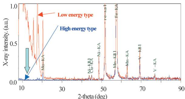
Fig. 3. Comparison between the high-energy-type and the low-energy-type polycapillary lenses.
