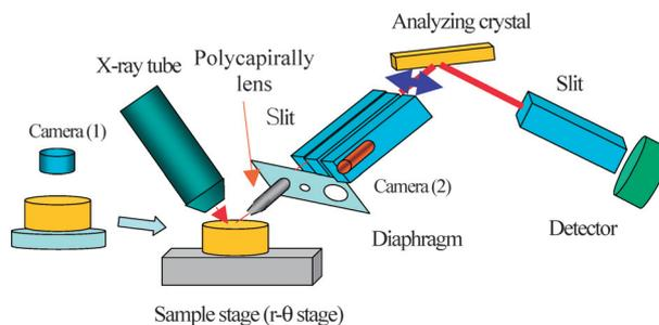
Fig. 2. Schematic diagram of the X-ray optics for the newly developed Rigaku WDXRF spectrometer.
