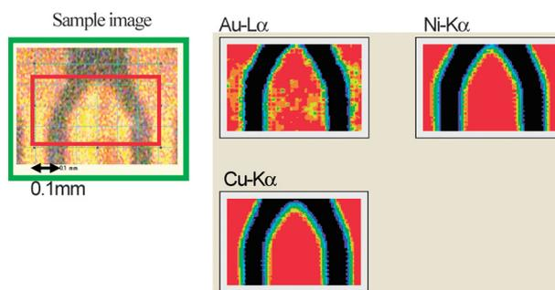
Fig. 7. Mapping analysis result of Au-L $\alpha$ , Ni-K $\alpha$  and Cu-K $\alpha$ .
