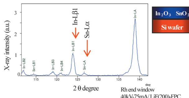
Fig. 8. WDXRF Spectrum showing In-L and Sn-L lines.
