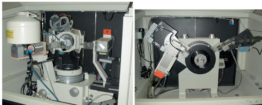
**Fig. A1.** 4-axis (base  $\theta$ - $2\theta$ ) and 2-axis ( $\theta$ - $\theta$ ) goniometers.
