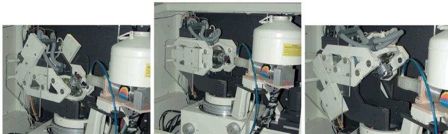
**Fig. A2.** 4-axis unit: Goniometer movements for  $\chi$  tilting and symmetric diffraction ( $\Omega=2\theta/2$  always). Left to right  $\chi$ :  $-55, 0, +55^\circ$ .
