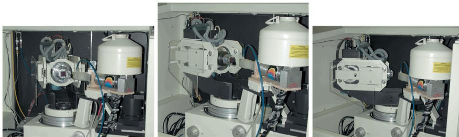
**Fig. A3.** 4-axis unit: Goniometer movements for  $\Omega$  tilting and asymmetric diffraction ( $\Omega \neq 2\theta/2$ ). Left to right  $\Omega$ :  $25.9, 70.9, 115.9^\circ$  corresponding to  $\Psi$ :  $-55, 0, +55^\circ$ .
