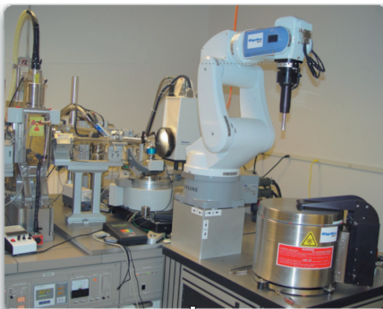
Fig. 1. A photograph of the ACTOR/Saturn92 system at UGA used in the experiments described. Briefly, the system consists of an FR-D Cu rotating anode, Osmic CMF15-50Cu8 (MaxScreen) optic, AFC9 goniometer, ACTOR automounter and Saturn92 detector.
