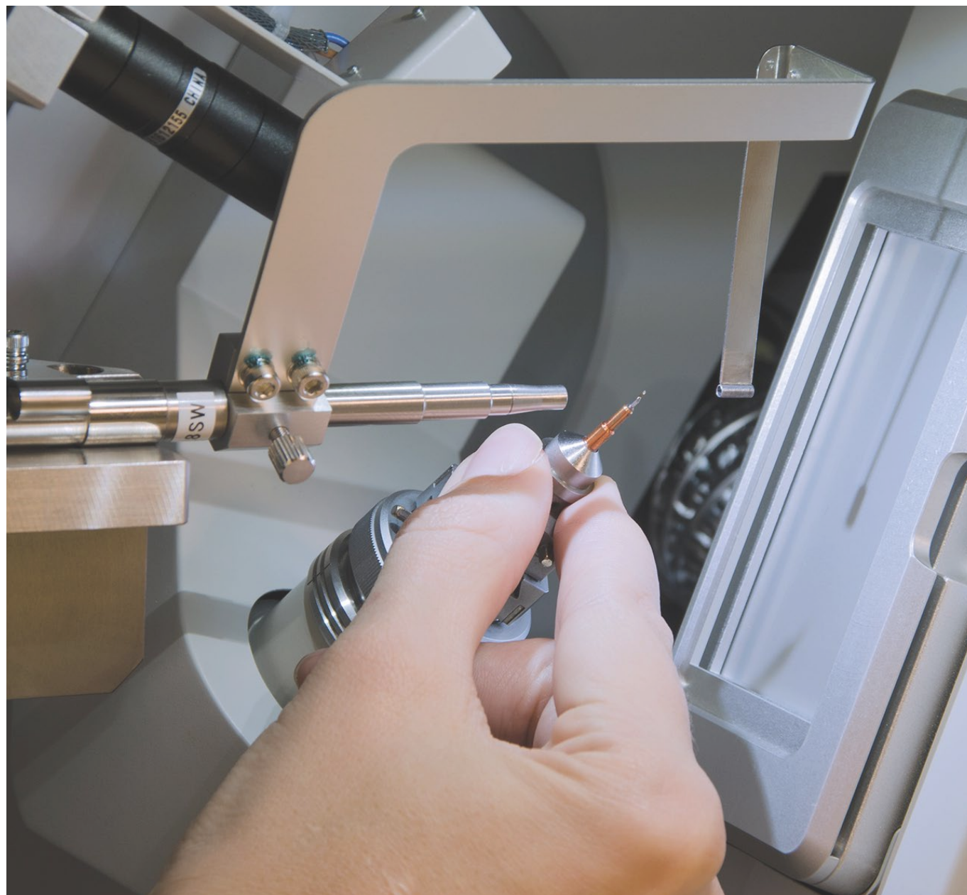
Mounting the crystal on the goniometer head.
