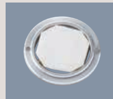
Alumina Intensity Standard Holder for Quantitative Analysis for Asbestos
