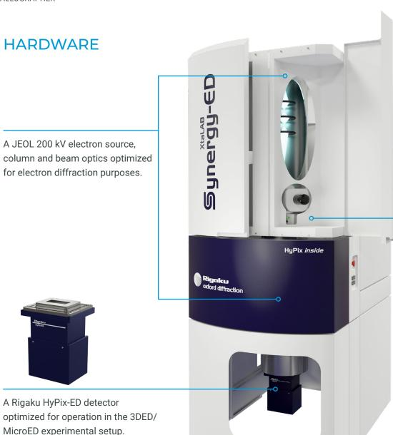
A sample stage allowing x, y, z sample alignment and rotation (tilt) about a single axis. A cryo option is available.
