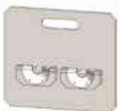
Film thickness direction Cell 2 slots Film specimens can be mounted in either portrait or landscape orientation
