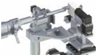
Sample Observation Camera A camera for sample observation that observes samples from the direction coaxial to X-rays.
