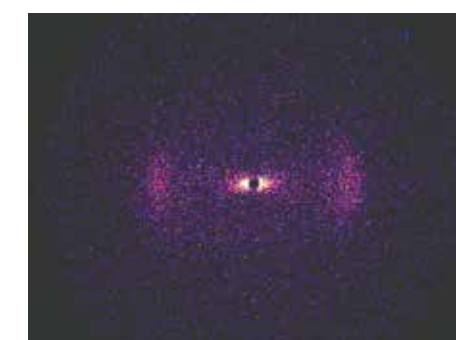
Measurement Results of a Single Carbon Fiber Evaluation of Fiber Orientation and Crystallinity
