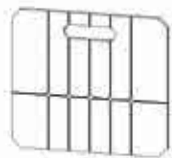
Standard Cell 5 slots (Hole diameter: φ 2 mm)
