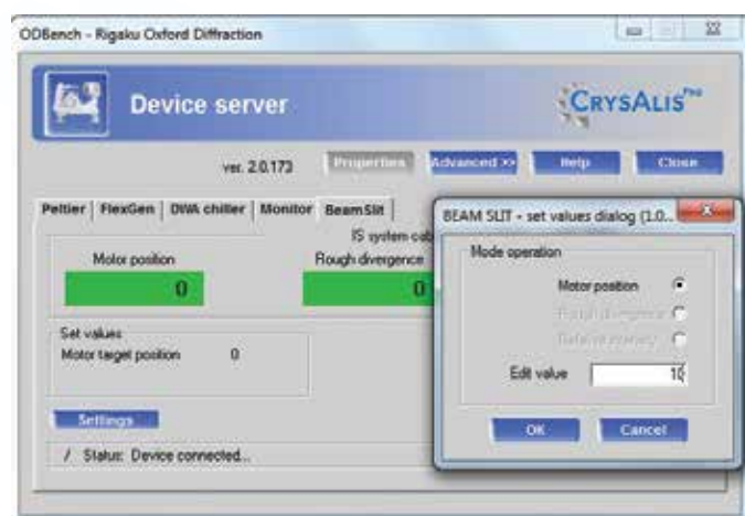
Software control of the slit assembly means that optimization of the divergence angle can be quickly carried out without the need to swap hardware or enter the radiation enclosure.
