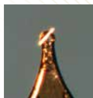
An image of the long axis crystal mounted on a MiTeGen loop.
