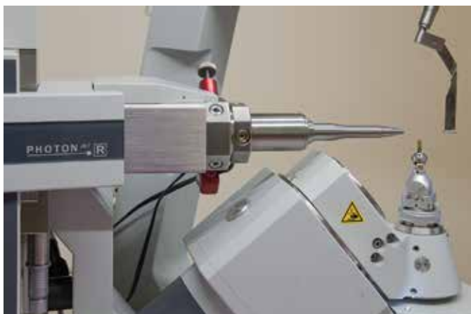
The Synergy slit assembly is integrated into the collimator holder and is controlled by the software package, CryAlis Pro .
