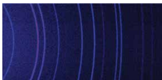
2D diffraction image measured in XRF suppression mode
