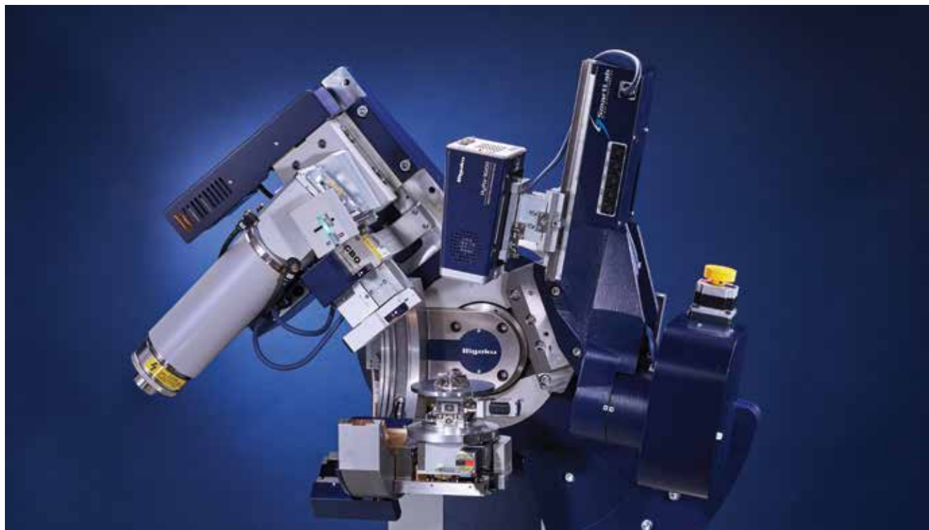
Residual Stress measurement optical configuration
