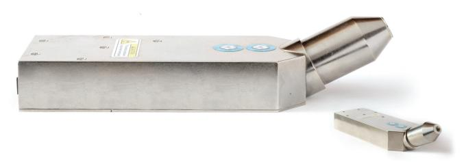
**Model M54:** 50 kV, 4W X-ray Monoblock - The M54 x-ray monoblock is a fully integrated miniature 50 kV, 4W x-ray generator designed specifically to be used as component of a handheld, portable, or benchtop x-ray instrument. The source includes a miniature sealed x-ray tube with a transmission-type end window, a high voltage power supply, and control electronics contained in a compact grounded enclosure.
