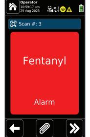
ready handheld Raman tool to also provide trace analysis of narcotics and explosives. With the addition of QuickDetect™ Technology, users are provided automated colorimetric results for the detection of non-visible trace amounts in seconds.
