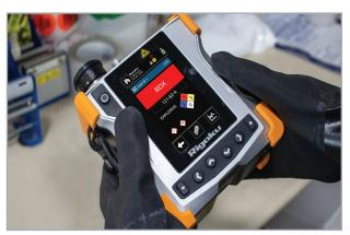
The Rigaku 1064 nm Raman analyzer displaying a result for RDX.
