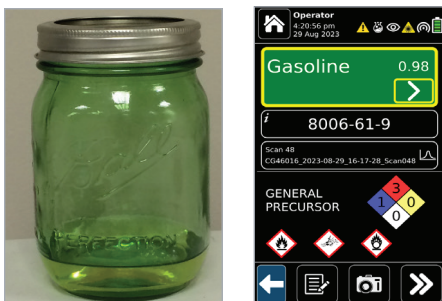
Figures 1 and 2. Analysis of gasoline through colored glass using a Rigaku CQL handheld analyzer.
