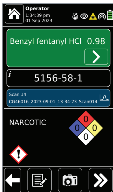
Examples of fentanyl precursor chemical results from the Rigaku CQL Series of handheld Raman analyzers.
