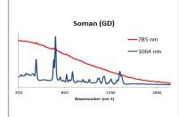
Figure 4. Raman spectra of munitions grade soman (GD) collected at 785nm (red) and 1064nm (blue).
