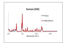
Figure 2. Pure (blue) and munitions grade (red) spectra of soman (GB), collected at 1064nm.
